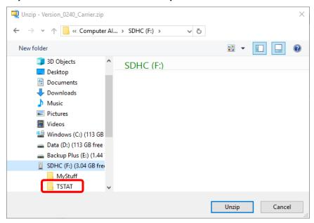
Verify that the files, including the BINF0380.hex file, have been extracted into the TSTAT folder of the MicroSD device. Note that the "USER" folder is where the photo and schedule files would be stored.
