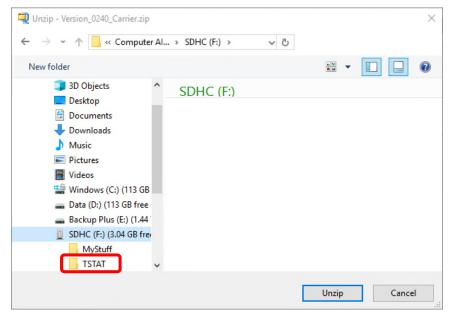
Verify that the files, including the BINF0361.hex file, have been extracted into the TSTAT folder of the MicroSD device. Note that the "USER" folder is where the photo and schedule files would be stored.
