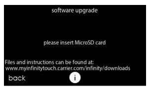
If the .hex file is stored properly on the MicroSD device, this screen will appear. If the screen says, "Please insert MicroSD Device", remove the MicroSD device and re-insert. If it still does not show the screen, below, go back to the download part and retry.
