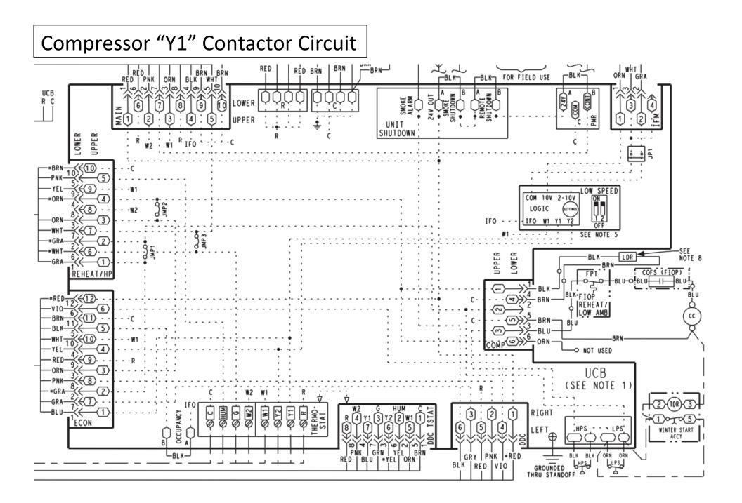
On the 48FC Series - Subcooling and **Hot Gas Reheat Dehumidification** Mode is energized through the thermostat (HUM) connection on main control circuit board.
