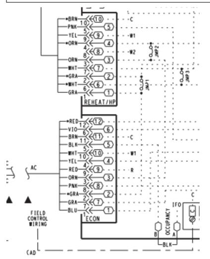
When HumidiMiZer Reheat board is added to a system. Jumper 1, 2 & 3 will be cut and removed.
