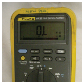
Fig. 23 – Checking NTC Circuit for Grounded Condition
