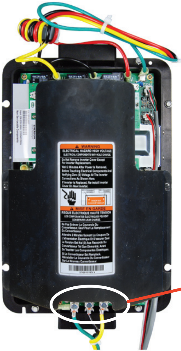
Fig. 26 – Measuring Input Voltage (VAC) to Drive L1 & L2
