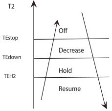
Fig. 23 - Evaporator Coil Temperature Protection
