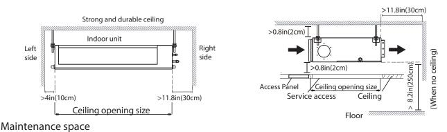
Fig. 3 – Installation Clearances
