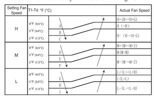
Fig. 18 - Indoor Fan Running Rules
