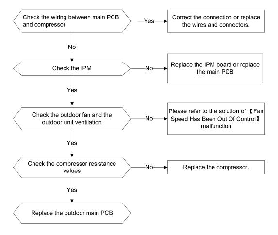
Outdoor IPM module temperature sensor malfunction diagnosis and solution (P7)
