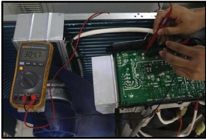
Fig. 39 – Measure the DC voltage
