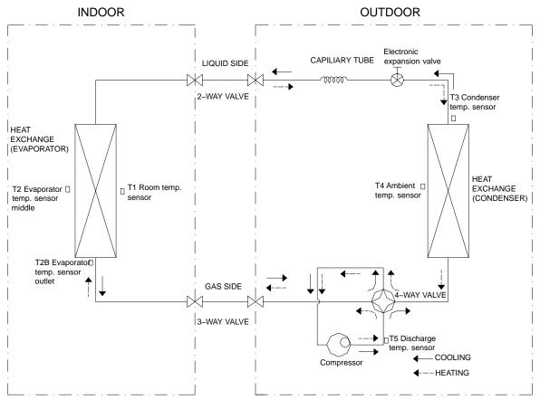
Fig. 12 - Refrigerant Cycle Diagram
