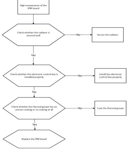
Fig. 41 - Troubleshooting - High temperature protection of IPM board diagnosis and solution (P2)
