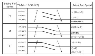
Fig. 20 - Indoor Fan Running Rules
