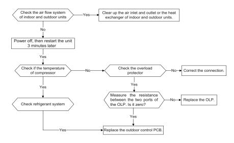
Fig. 40 - Troubleshooting - High temperature protection of compressor top diagnosis and solution (P2)
