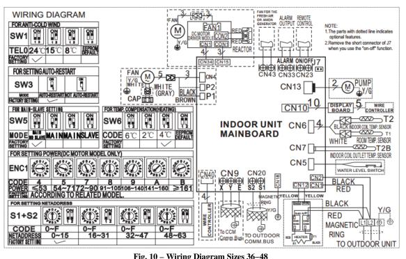
Fig. 10 – Wiring Diagram Sizes 36–48
