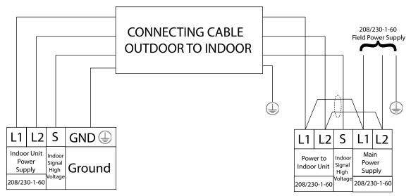
Fig. 5 – Connection Diagrams 9–24
