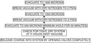
Fig. 16 - Triple Evacuation Method
