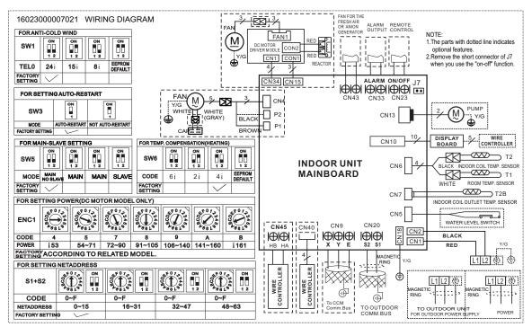
Fig. 11 – Wiring Diagram Size 58
