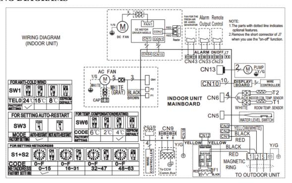
Fig. 9 – Wiring Diagram Sizes 9K – 24K
