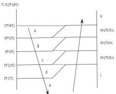
Fig. 19 – Indoor Fan Running Rules
