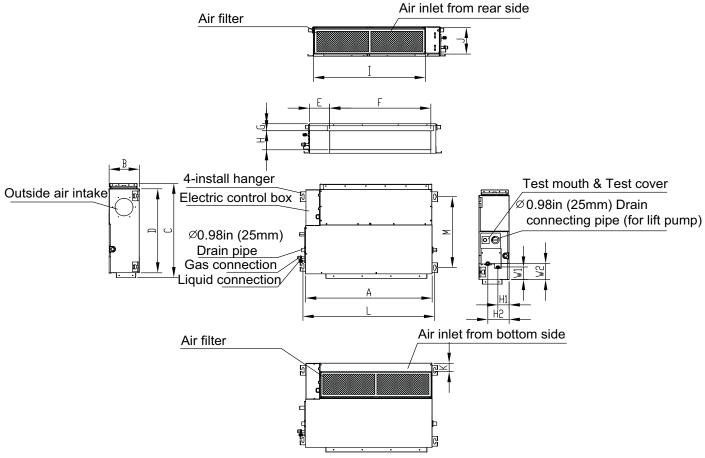
Fig. 1 – Indoor Unit Sizes 9K – 48K
