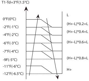
Fig. 21 - Auto Fan Action in HEATING Mode
