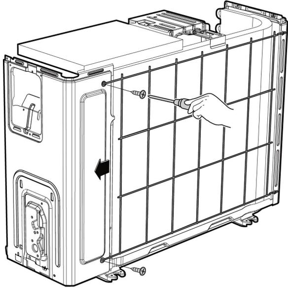
7) Remove the right panel screws (6) and then remove the right panel.
