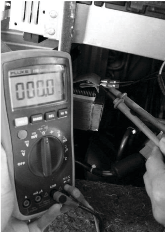
Fig. 32 —Reactor resistance test
