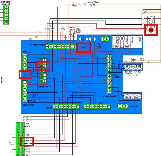
Low Voltage – 1<sup>st</sup> Stage Cooling
