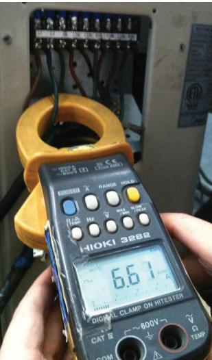
Fig. 66 — Test the voltage
