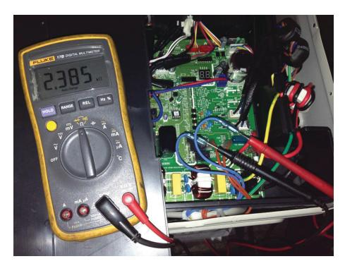
Fig. 72 — Test the Resistance
