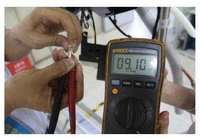
Fig. 51 — Check the Sensor Value
