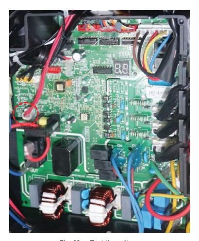
Fig. 62 — Test the voltage
