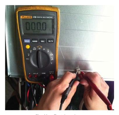
Fig. 63 — Test the voltage
