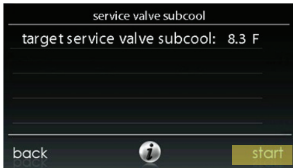
Fig. 10 – Service Valve Subcool Target Value
